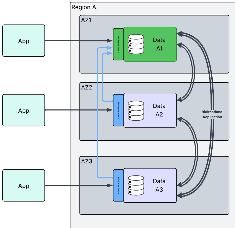
In this diagram, you can see the applications connecting to the PGD cluster through the Connection Manager ports. The Connection Manager is responsible for routing the read and write transactions to the appropriate nodes in the group. The write leader is responsible for handling all write transactions and is shown in at the top in AZ1 in green.
